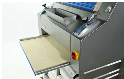
Stainless steel wool felt covered collection tray on slides.
