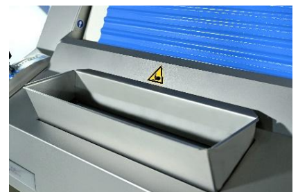
Hinged stainless steel safety hopper at dough infeed.
