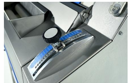
Handy placed levers for accurate positing and adjusting of infeed and belt rollers.
