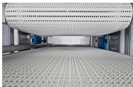
Adjustable upper conveyor belt for free baked and round bread.
