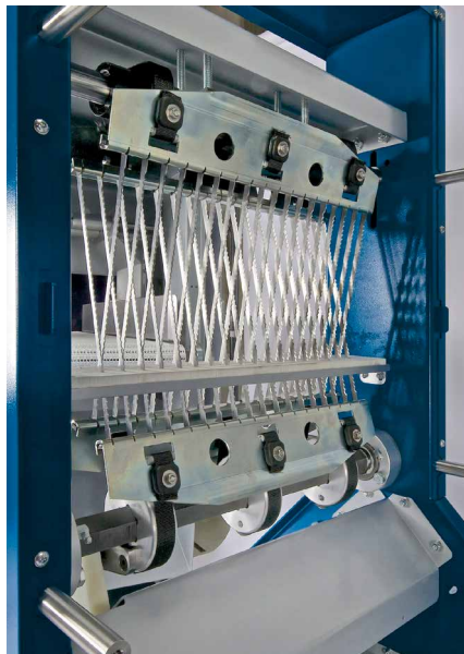
Unique and proven cross-slice system with angled blades that last up to three times longer.
