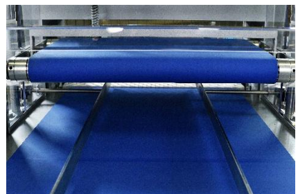
Double infeed belt with electronic variable speed.
