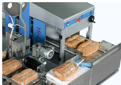
After slicing of the bread, a bag blowing device automatically opens the plastic bag.
