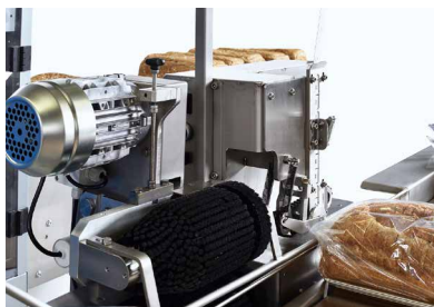
Brush roll for flattening the bag before closing.
