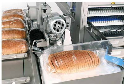
After slicing of the bread, a bag blowing device automatically opens the plastic bag.
