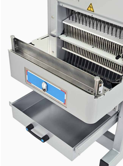
Easy accessible crumb tray collector at the front side for easy cleaning.
