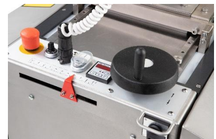
The SLIM dough divider is designed for daily use. The machine is equipped with electronic speed control and piece counter.
