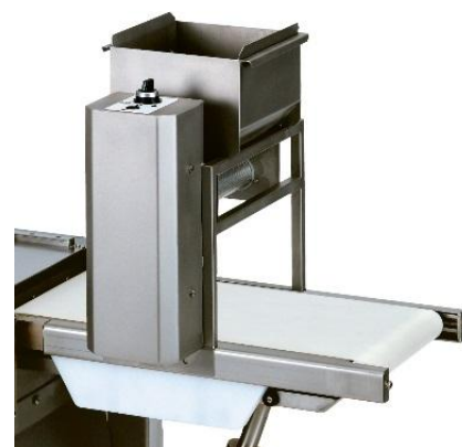
Stainless steel automatic flour duster with precise continuous or interval flour dosage (option).
