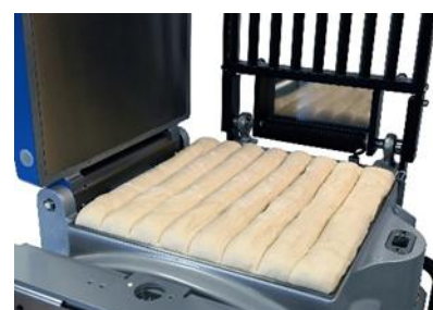
Forming plate and forming grid for 6, 8 or 10 baguettes.
