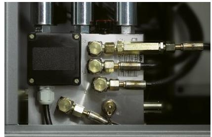
Adjustable hydraulic pressure regulation for extra flexibility and a wide range of dough types.
