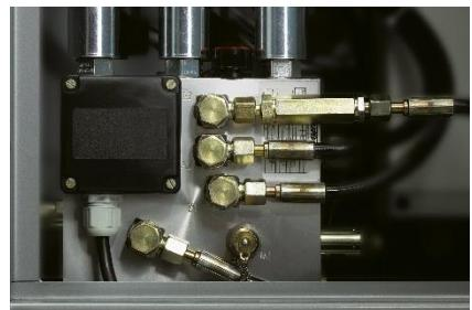
Adjustable hydraulic pressure regulation for extra flexibility and a wide range of dough types.
