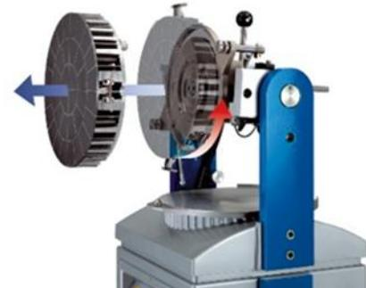
Interchangeable dividing disc (within 5 minutes) offers increased flexibility, a work range of 0.6-15.5 oz. and tilts forward for easy cleaning.
