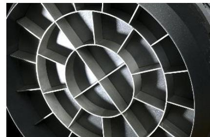
Anodized aluminium dividing disc and stainless steel knife require minimal flour for dividing and are hygienic in use.
