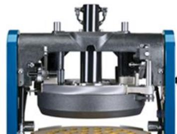
Low-pressure dividing system respects the dough and requires no physical effort from the operator. The DR Robot is equipped with reliable and proven electronics and silent, specially engineered long life hydraulics with low operating temperature.
