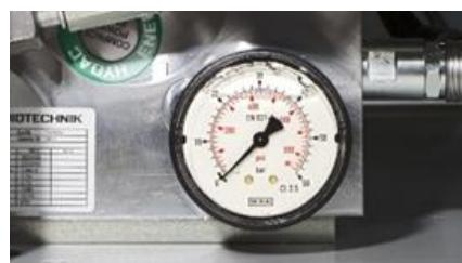
Standard on Variomatic and an interesting option on other DR Robot models; variable pressure regulation for any dough type.
