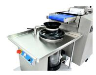
If required, rounder can be easily disconnected from the portioner and used as a stand-alone unit for up to 2400 (1 - 60 oz.) pieces per hour.
