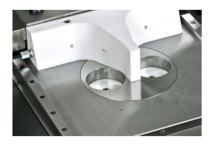
High grade stainless steel vacuum cylinder available with single or double piston.
