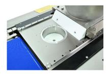
Healthy hygienic; no dough remains in the vacuum chamber which makes the SLIM easy to clean and perfectly suitable for quick changing of dough types.
