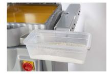
Handy removable flour tray with top cover which can be fixed on various positions on the machine.
