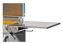
Stainless steel working table on left or right side which can be folded down completely.
