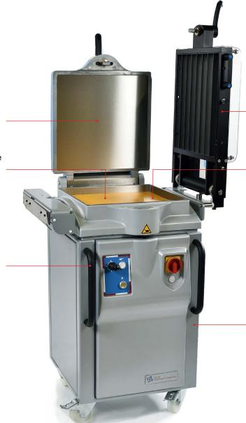
Solidly constructed grid support is closed, locked and unlocked in one simple natural movement.
