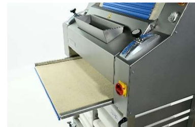
Extendable collection tray with easy exchangeable wool felt cover.
