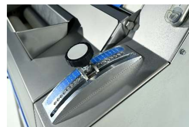
Handy placed levers for accurate positioning and adjusting of infeed and belt rollers.
