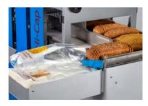
After slicing of the bread, a bag blowing device automatically opens the plastic bag. Sliced bread is inserted manually in one natural movement, saving considerable time.
