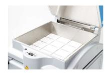
High grade stainless steel dividing knife for weight ranges from 120 to 3340 gr.
