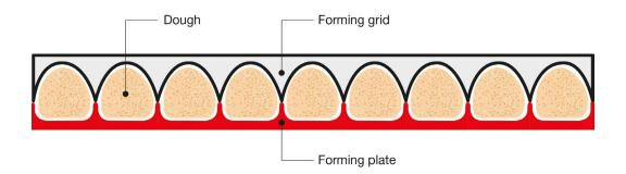
Designed for preparing well-rounded, fluently shaped baguettes without outside markings.
