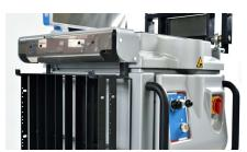
Storage hooks for max. up to 3 grids on one or both sides of the machine.
