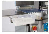
Handy removable flour tray with top cover which can be placed on 4 various positions on the machine.
