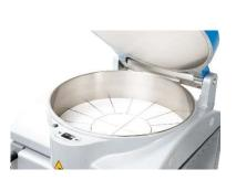
Dividing disc with stainless steel knife and ring around the dough tub make the Robocut robust and hygienic.
